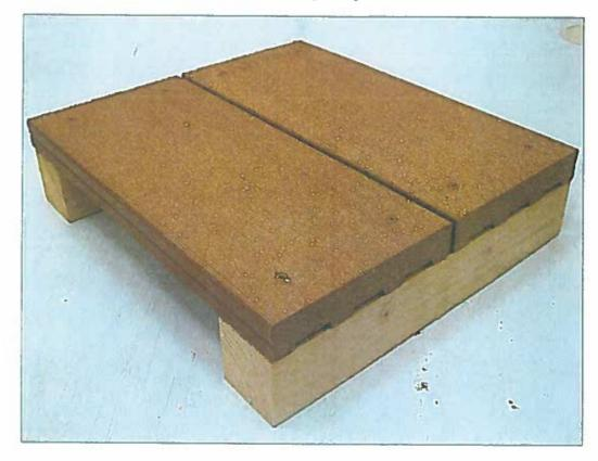
Mean Rz Surface Roughness: 31.0µm Pendulum Test Values:
